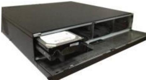
③ Insert the HDD to the clip and adjust the handle of the HDD to secure it.
