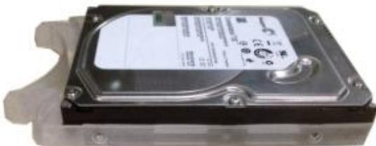
① Line up the one side of the handle to the HDD (The side of no port)
