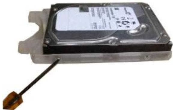
② Use screwdriver to fix the handle on the HDD.
