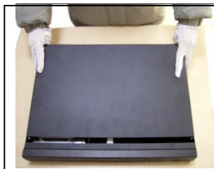
② disassemble the cover
