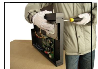
③ fix the screw of hard disk
